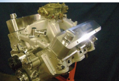
750hp pump gas aluminum MR-1A block
