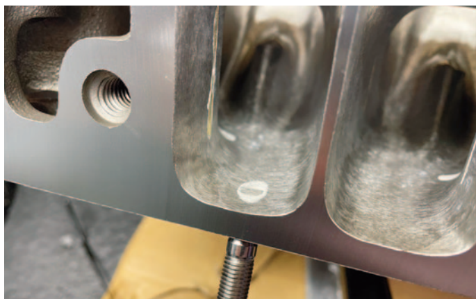
The roof of the ports were raised so much that on some ports, the valve cover retainer bolt holes were exposed. The fix was easy, however, with studs and some carefully-applied JB weld to seal them in.
