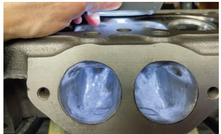
As for the exhaust side of the heads, factory IV castings flow well — obviously. But Nitemare's ported ones flow sooooo much better: 245 cfm, to be specific — as well as factory intake port flow! — and far better than factory ports at about 180 cfm.
