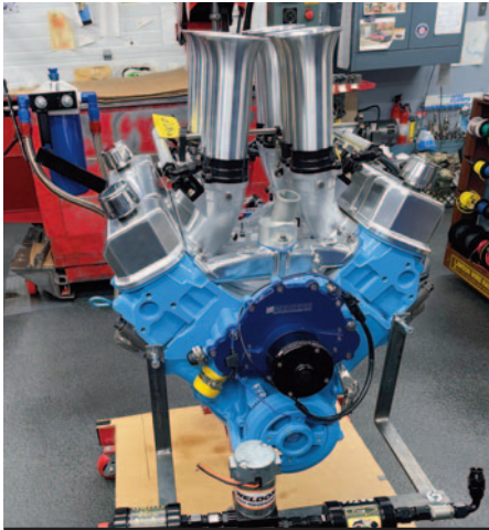
Here's the Kinsler setup being test-fit to the engine, along with some temporary bracketry to hold the fuel filters and pump when the engine goes to the dyno.
