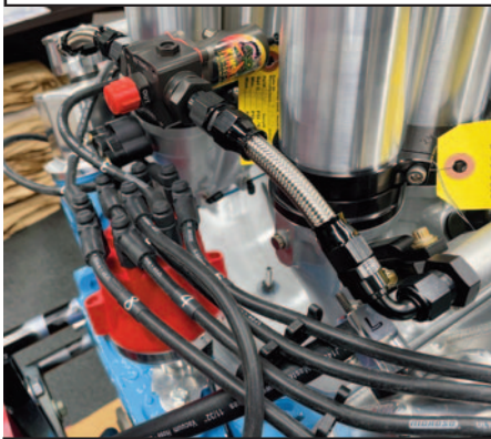
At the back of the engine fuel flows from the rails to a common pressure regulator that then allows fuel to return to the tank. This helps prevent fuel percolation since fuel doesn't dwell in the rails absorbing heat, and obviously the pressure regulator ensures the injectors get the pressure they need to produce an effective spray pattern. The MSD distributor was used for mock-up purposes and break in with the carb setup; a Holley dual-sync unit is more compatible with the engine's control unit and was used for dyno testing.
