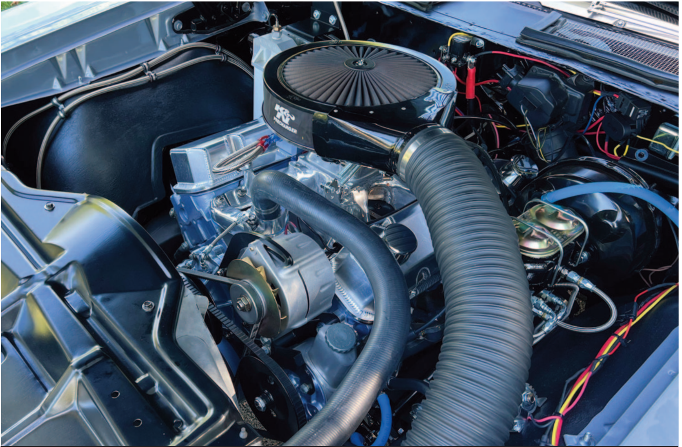
While the hood scoops provide cool air into the engine compartment, The Cleener has real ram air drawn from an empty headlamp bucket through a gargantuan hose direct to the K&N air filter assembly.
