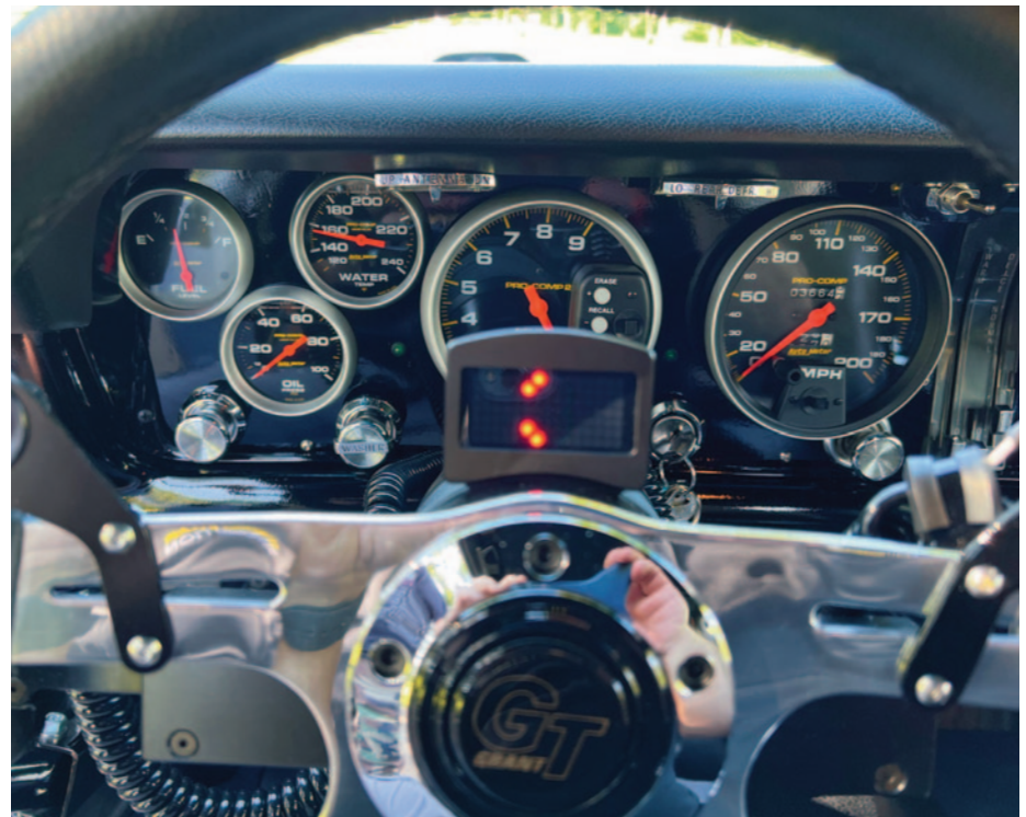
Magro outfitted the factory dash with enough Autometer gauges to keep tabs on a nuclear powerplant ... all neatly arranged in a factory dash.
