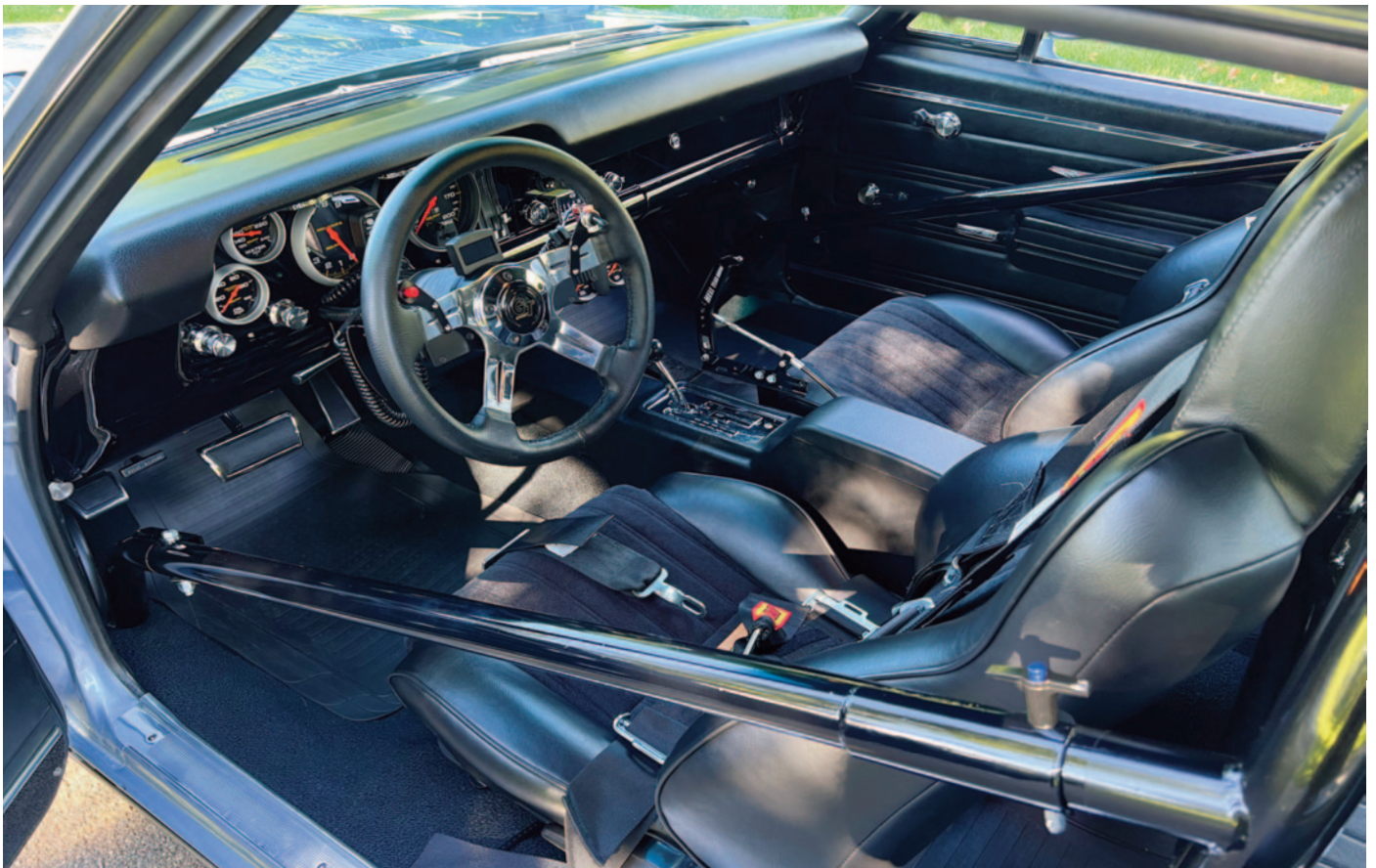
With the doors shut, you'd almost never notice that the interior sports a roll cage, upgraded seats and five-point belts, and one of Magro's favorite items: a factory Hurst DualGate shifter controlling a beefed up 4L80 automatic transmission.
