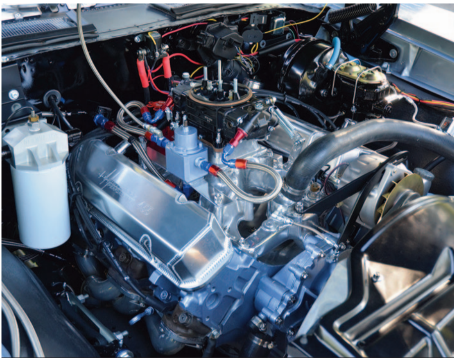
The Cleener's engine is a 455 HO block with heavily-ported Ram Air IV heads making 664 horsepower and 545 pounds-feet of torque. Note the lack of nitrous, a turbo, or a blower.
