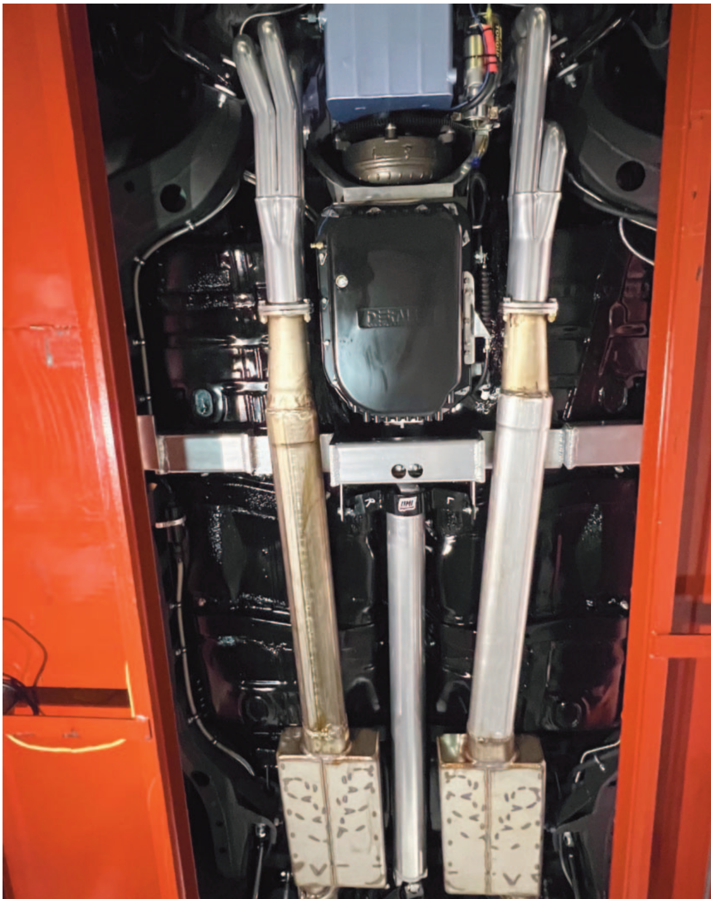
The undercarriage is clean enough to eat off. The frame was powder-coated, the ceramic-coated Doug's Headers flank the engine, a 4L80 automatic, and feed into 3.5-inch oval pipes and SpinTech mufflers.
