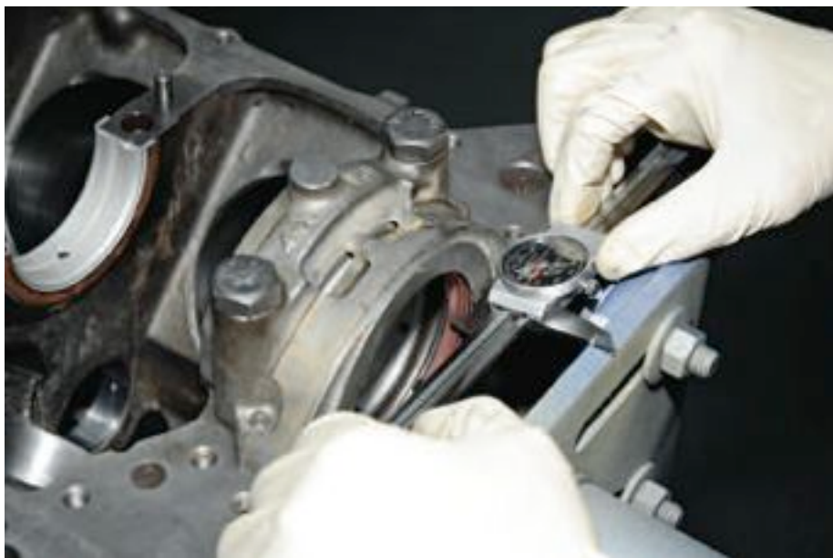
The devil's in the details. A proper Pontiac V8 rebuild involves meticulously measuring everything and either select-fitting parts or making minute adjustments to optimize clearances, a process often referred to as "blueprinting." The reward for all the tedious labor is an engine that can produce more power and will last longer.
