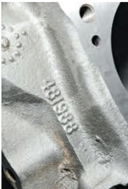
Speaking of matching numbers ... Pontiac blocks have lots of numbers that tell us what it is and what it originally came in. This is the casting number: 481988, which tells us that it's an early-1970s 400. The clock-like dial near the top-left of the photo indicates the hour at which the block was cast: 7 am or 7 pm, in this case. To know which, we have to look elsewhere ...
