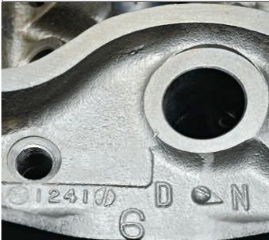
The surface adjacent to the distributor hole contains a wealth of information about a Pontiac block: "1241" is the date code: September, 24, 1971, so for a 1972 model year vehicle. The arrow pointing to "N" tells us that it was cast during the night shift ... so the clock in the previous photo indicated 7 pm. Many blocks also feature a large two-digit code cast to the left of the distributor hole, to indicate the year it was produced, but this one clearly does not.
