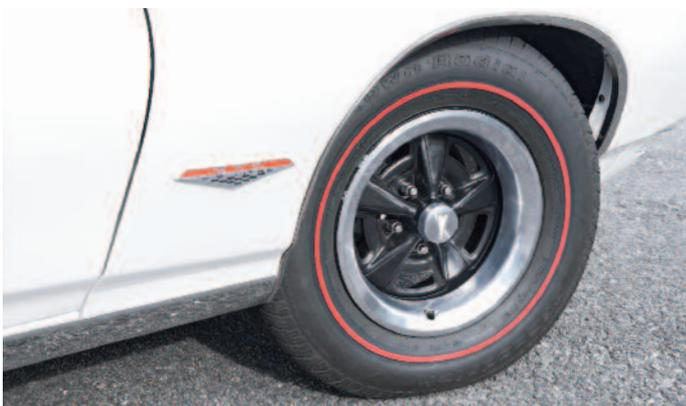
**As with the drivetrain, the Wolfs' GTO received a few stealthy upgrades in the chassis department, the most noticeable of which are the slightly-upgraded 15-inch Rally II wheels wearing BFG Silvertown redline radials. Between the wheels are a host of Hotchkis Suspension springs, shocks, swaybars, and bushings to improve the Goat's handling.**
