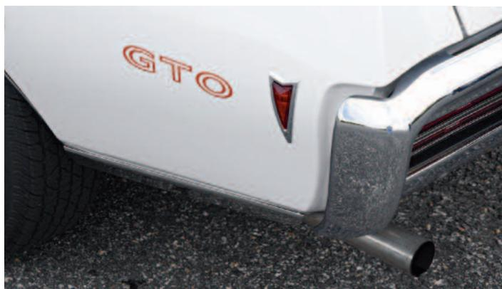
**All the bright trim like marker light bezels and the rear bumper were either restored or replaced, along with decals, emblems, and other bits to bring the body back to factory-type condition. Any of the modifications chosen – like the blacked out grilles and wheels – can be easily returned to stock, if Ed ever gets the urge in the future.**
