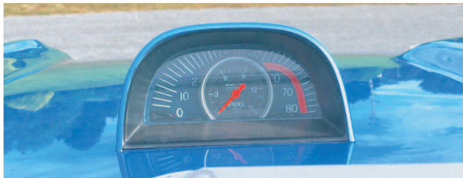
Nitemare modified the stock Pontiac hood tach – which are notorious for being slow and inaccurate – to house a fuel pressure gauge, so Richard can keep tabs on the Holley electric pump's output.
