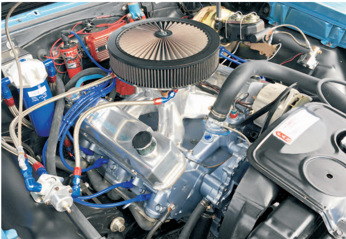
This is the fourth engine that's been in Richard's GTO, since he's owned it. This one's a Nitemare Performance crate motor that puts out 500 horsepower! A Tremec five-speed and 3.90:1 Safe-T-Track transmit the power to the pavement.
